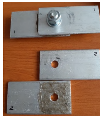
Fig. 4. Application of functional composite material to contact surfaces
