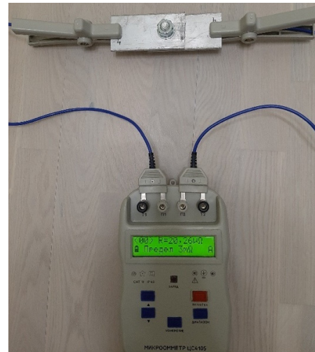
Fig. 5. Measuring the resistance of the contact connection
