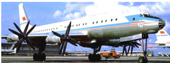
Fig. 9. Soviet long-distance (intercontinental) turboprop four-engine passenger aircraft of the type Tu-114 developed by A.N. Tupolev (1958) [6]
