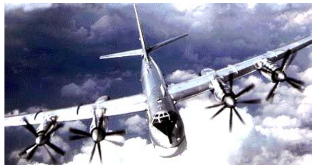
Fig. 8. Soviet turboprop four-engine strategic bomber of the Tu-95 type («Atomic Bear» in the terminology of NATO countries) developed by A.N. Tupolev and his fellow aircraft designers at the Design Bureau-156 (1956) [7, 8]
