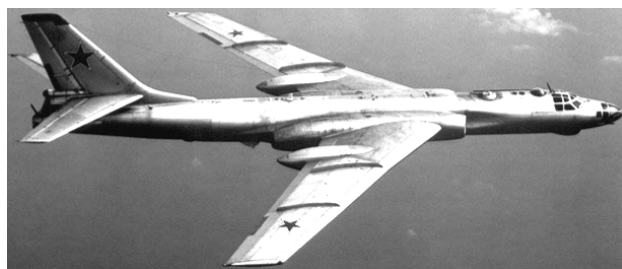
Fig. 5. Soviet jet twin-engine long-range missile-carrier bomber of the Tu-16 type («Russian badger» in the terminology of NATO countries) developed by A.N. Tupolev (1953, chief designer of the machine – D.S. Markov) [5]
