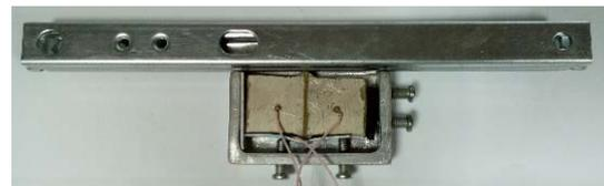
Fig. 8. Experimental sample of linear piezoceramic motor
