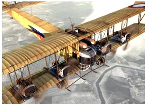
Fig. 3. Four-engine bomber «Ilya Muromets» (S-22) of military transport purpose developed by I.I. Sikorsky (1913, Saint Petersburg, Russia) [2]
