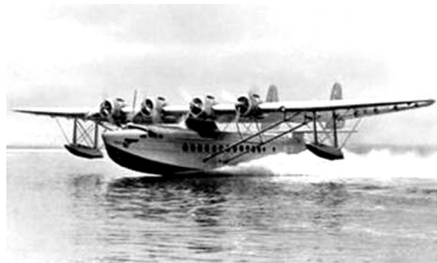
Fig. 6. Four-engine long-range fifty-passenger amphibious aircraft of type S-44 developed by aircraft designer I.I. Sikorsky (1937, USA) [2]
