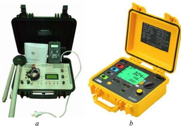
Fig. 4. Devices for monitoring the state of the GD:
