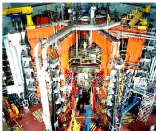
Fig. 6. General view of the world's largest operating thermonuclear tokamak JET, created by Euratom and located near Oxford in the nuclear research center Culham Lab (1997, Abingdon, UK) [18]
