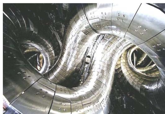
Fig. 8. General view of a working vacuum metal chamber with a hot plasma of an experimental thermonuclear stellarator installation curved in the shape of complex 3D serpentine configuration («crumpled donut») [9]
