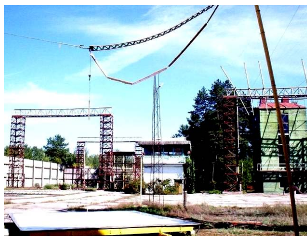
Fig. 14. General view of a superhigh-voltage ohmic voltage divider of the ODV-2,5 type for a rated voltage of \pm 2.5 MV, connected in the CVPG discharge circuit to a two-electrode «needle-plane» system with an air gap length of 3 m (the upper steel rod-electrode of this electric discharge system is located at the center of its lower flat electrode made of thin galvanized steel with a plan size of 5 m \times 5 m) [23]
