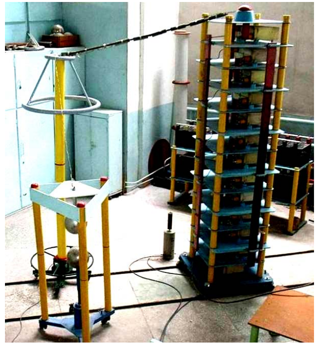
Fig. 11. General view of the high-voltage test stand of the R&DPCI «Molniya» of the NTU «KhPI», on the test field of which mobile generator of pulsed voltages of the type GIN-1,2, the divider of the type ODV-1 and standard measuring balls with a diameter of 250 mm are placed [17]
