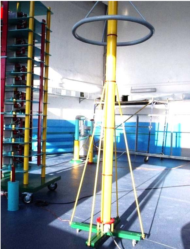
Fig. 10. General view of a mobile superhigh-voltage ohmic voltage divider of the type ODV-1,2 at a rated voltage \pm 1.2 MV, located at the factory test field of a high-voltage test stand SVI-1,2, designed to determine in the laboratory conditions the pulsed electrical strength of polymer insulation of its own production (enterprise ES «Polymer», Bakhmut city, Ukraine, 2006) [9, 17]
