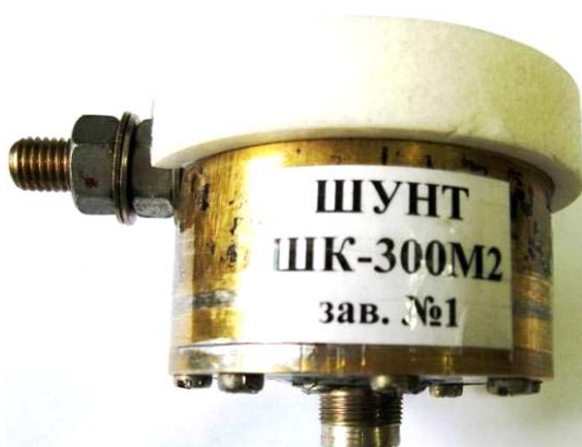
Fig. 2. External view of the improved coaxial shunt type SC-300M2 designed to measure in the coordinated mode of operation of its cable signal transmission line in the micro- and millisecond ranges of current pulses of artificial lightning with amplitude up to \pm 220 kA in the high-current discharge circuit of high-voltage LCG with their integral of action up to 15 \cdot 10^6 J/Ω [11]
