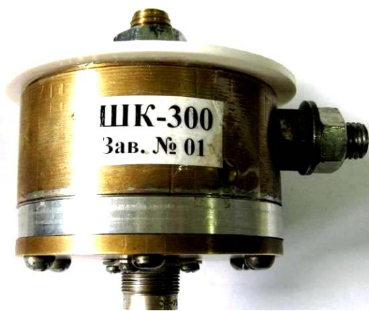
Fig. 1. External view of the improved coaxial disk shunt type SC-300M1, intended for measurement in the micro- and millisecond ranges of damped sinusoidal and aperiodic current pulses of artificial lightning with amplitude up to \pm 220 kA in the high-current discharge circuit of a powerful high-voltage LCG with their integral of action up to 3 \cdot 10^6 J/Ω [10]
