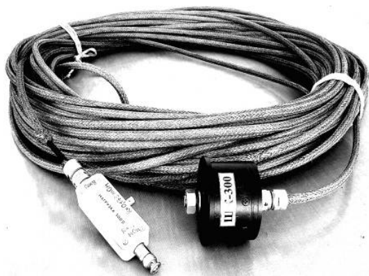
Fig. 4. External view of the SC-300M1 measuring shunt connected to the input of an additionally shielded coaxial RF cable of the RK 75-7-11 type with a length of 70 m, the output of which is connected to a shielded matching voltage divider of the type SDN-300 with two output coaxial connectors 1:1 and 1:2 for the coordinated connection of the measuring channels of the three DSO (for example, Tektronix TDS 1012 series) to them, while simultaneously registering of three components of the total current pulse of the artificial lightning in the high-current discharge circuit of the LCG with different ATPs [6, 10]
