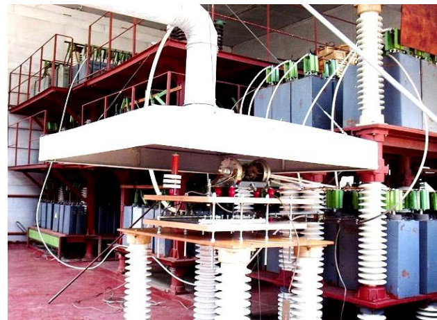
Fig. 1. General view of a powerful high-voltage high-current generator of artificial lightning current of the type УИТОМ-1 (in the foreground there is a desktop with a high-voltage three-electrode air controlled switch with steel electrodes for a voltage of \pm 50 kV and pulsed sinusoidal lightning current up to \pm 220 kA, a tested sample of the skin of an aircraft and an air drawing system, and in the background – separate high-voltage pulse current generators for the corresponding current components A, B, C, C^* and D ) [11]
