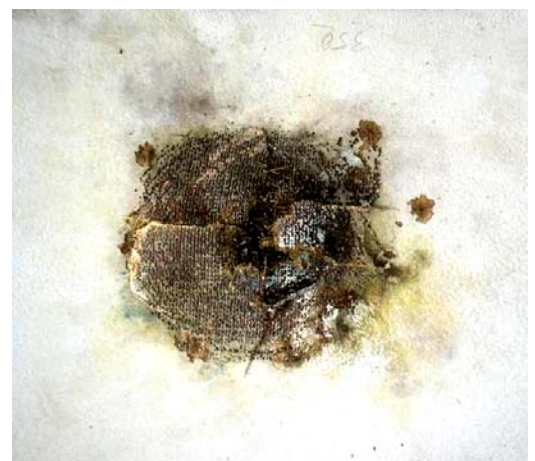
Fig. 8. General view of the damage zone with a diameter of up to 100 mm with a through burn in an experimental sheet specimen of 3 mm thickness of the composite plating of an aircraft tested in the high-current circuit of the powerful GCL of the УИТОМ-1 type, at a direct action on it of normalized by [7, 8] pulsed A - components of artificial lightning current [10]
