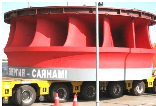
Fig. 5. General view of the carried to the HPP impeller to the HPP of a modern powerful radial-axial hydraulic turbine [7]
