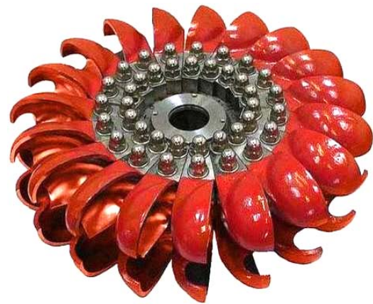
Fig. 7. Enlarged view of a new impeller of a modern powerful bucket hydraulic turbine before its installation in the machine room of a high-pressure HPP [10]
