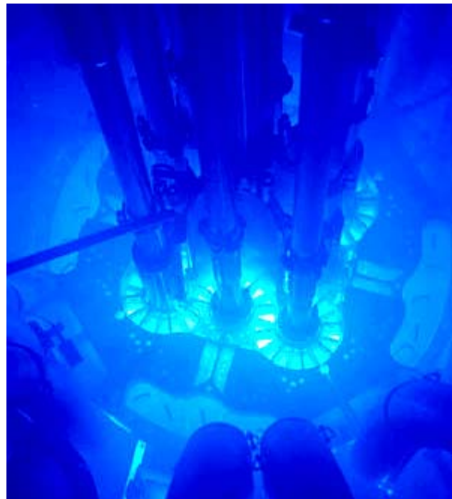
Fig. 5. The rarest view of active zone of the active research water-water nuclear reactor (in the active zone of this type of reactor there is clearly observed a blue glow caused by Vavilov-Cherenkov radiation) [2]
