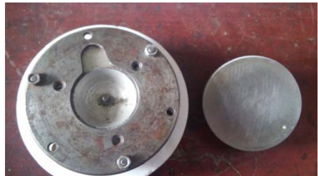
Fig. 2. Variant of stationary WCH with cover – electrode located near
