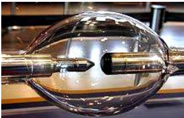
Fig 8. General view of a 15 kW xenon arc lamp used in a modern IMAX projector [15]
