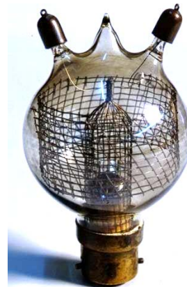
Fig. 2. General view of the first Russian powerful radio lamp «Babushka» («Grandmother») (Nizhny Novgorod Radio Laboratory, 1919) [9]
