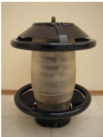
Fig. 9. External view of a high-voltage broadband voltage divider BДН -75 designed to measure DC, AC and pulse voltages of 110 kV class (the nominal value of the division factor is K_n = 10000 )
