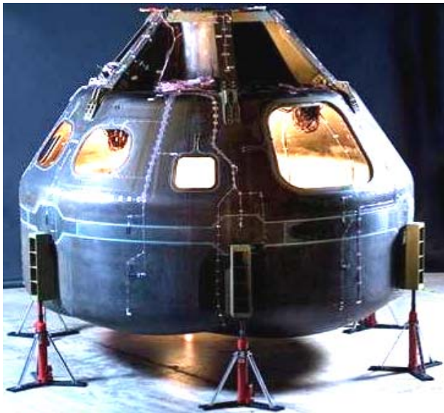
Fig. 5. The general view of the orbital compartment of the new spaceship Liberty (USA) made on 90 % of polymer composites and intended for the re-delivery of astronauts and scientific cargoes on board the ISS [17]
