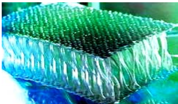
Fig. 2. General view of a fragment of the original glass fiber fabric of the type Parabeam 3D Glass fabric consisting of two woven horizontally placed parallel glass plates connected to each other by vertical glass worm and forming the so-called «sandwich-glass structure» [6]
