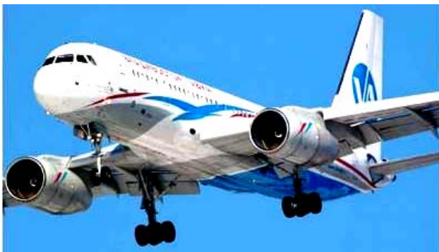
Fig. 3. The general view of a medium-haul passenger aircraft of the Tu-204 type (RF, 1990's) in which up to 25% of all parts of the glider were made of composites [14]
