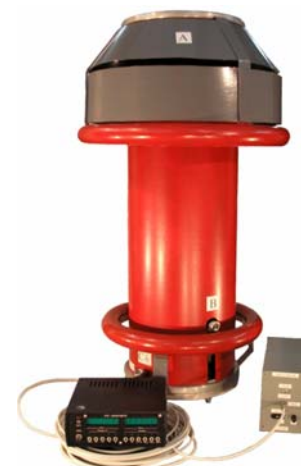
Fig. 8. General view of the set for measuring high voltage BBH-0,8-100M in the composition of a high-voltage arm, a low-voltage arm, a specialized digital voltmeter and connecting cables. The separate design of the low-voltage divider arm is due to the possibility of its adjustment and switching for the high-voltage measuring ranges 0.8-10 kV and 10-100 kV
