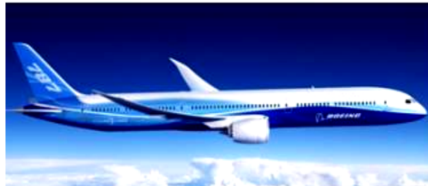
The general view of the main passenger aircraft of the type Boeing 787 Dreamliner (USA, 2015) the fuselage and wings of which were 90 % made of composites [14]
