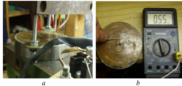
Fig. 10. Experimental installation for LPIEC research with a thin-walled steel framework (a) and temperature measurement process (b)
