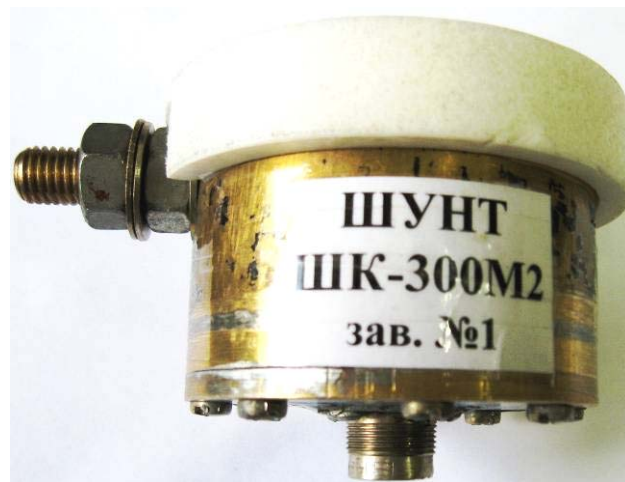
Fig. 1. General view of a coaxial shunt type IIIK-300M2 designed to measure on the screens of the DSO in an agreed mode of operation of its coaxial cable communication line of powerful current pulses of artificial lightning in a high-current discharge circuit of a high-voltage GCL with an integral of their action up to 15 \cdot 10^6 J/Ω
