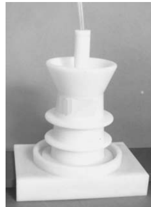
Fig. 10. Design of high-voltage overcurrent reed relay not requiring CT: 1 - main insulator; 2 - fixative plate; 3 - inside nut; 4 - semi-conductive cover; 5 - bushing; 6 - fixative nut; 7 - fastener; 8 - reed switch; 9 - high-voltage bus bar; 10 - epoxide compound
