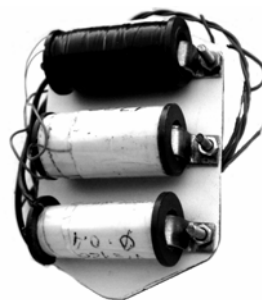
Fig. 4. The unit of inductive sensors for high current pulses
