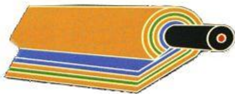
Fig. 12. Multilayered shielding of poly-sandwich developed by Belden
