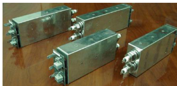
Fig. 17. Sealed power filters manufactured by Captor Corp. designed for AC and DC power circuits up to 100A ensuring effective EMP attenuation to not less than 100dB within the frequency range of 14kHz-10GHz
