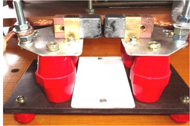
Fig. 3. External view of high-voltage two-electrode air switch type ВДБК-10 with graphite electrodes of rectangular shape for voltage up to \pm 10 kV used in the discharge circuit of the generator PCG-C [2]
