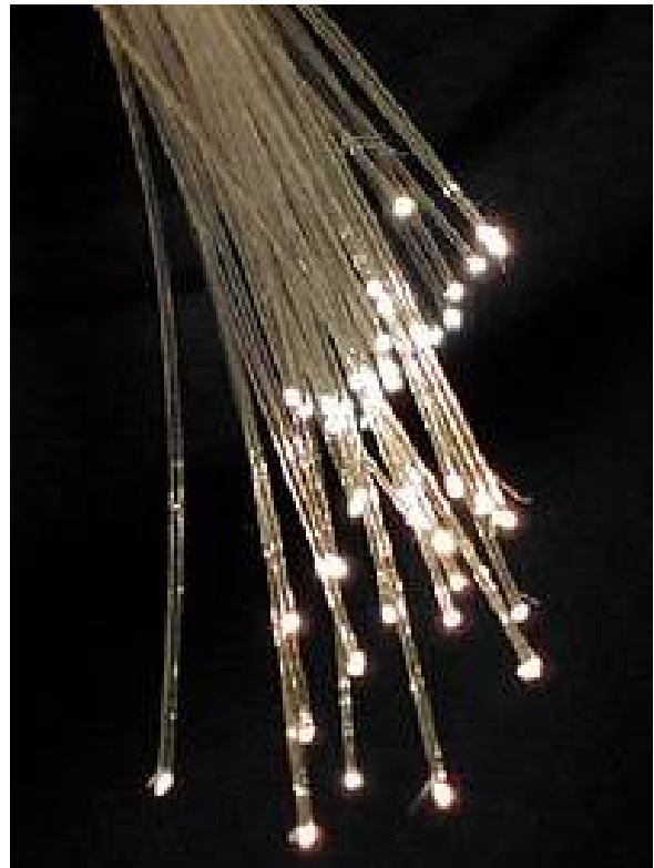
Fig. 16. External view of a fragment of a bundle of optical fibers with quartz filaments in a protective shell, effectively transmitting light pulses for long distances [22]
