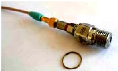
Fig. 14. External view of the piezoelectric sensor of pressure pulsations M101A06 by the PCB Company
