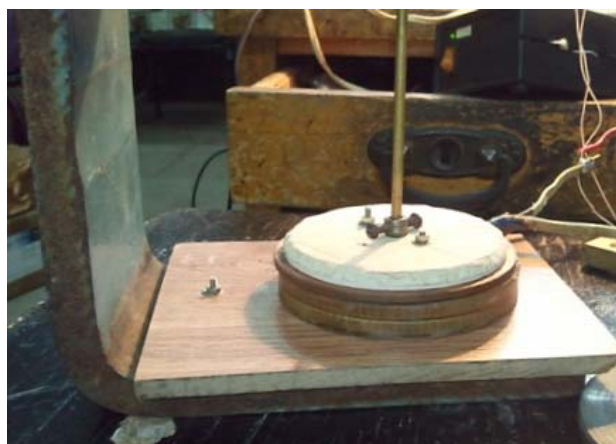
Fig. 18. General view of the experimental setup for investigations of LIEC working as an accelerator with ceramic power disk
