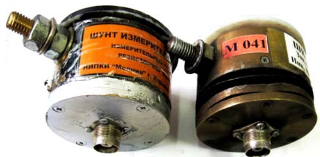
Fig. 4. General view of the measuring coaxial shunt type IIIK-300 before (left) and after (right) flow through it in high-current discharge circuit of the ГИТМ-10/350 normalized artificial lightning current aperiodic pulse temporal shape 15/315 \mu s with amplitude I_{mL} \approx 184 kA ( q_L \approx 81.3 C; J_L \approx 7.88 \cdot 10^6 A 2 ·s)
