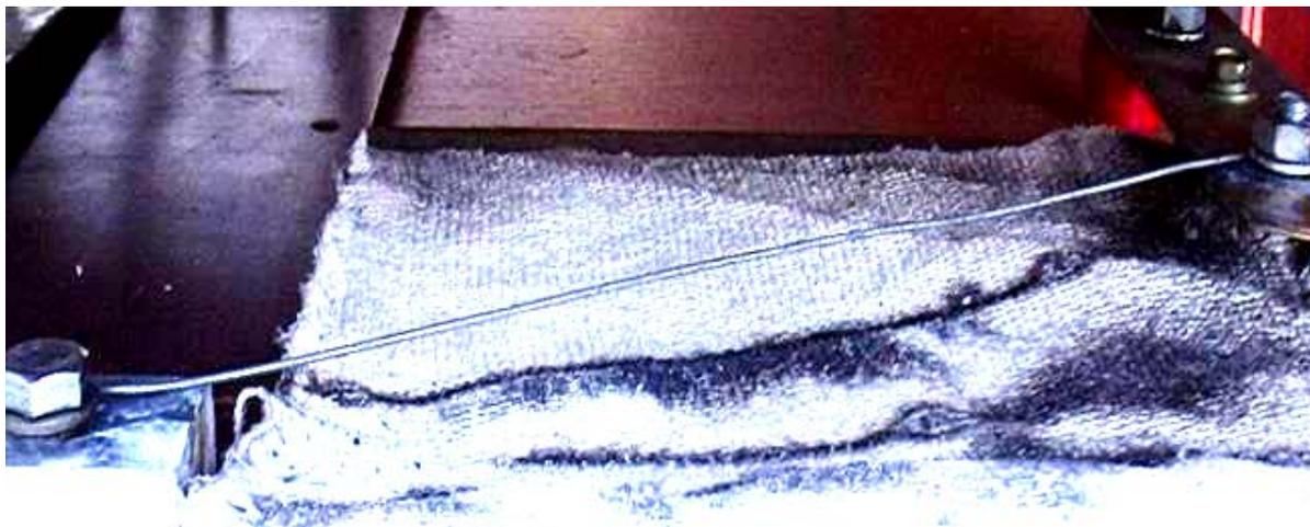
Fig. 2. General view of the continuous round galvanized steel wires ( $r_0=0.8$  mm;  $l_0=320$  mm;  $\Delta_0=5$   $\mu\text{m}$ ;  $S_0=2.01$   $\text{mm}^2$ ) included its ends by means of a bolted joint in high-power high-voltage discharge circuit GPC-C and placed on a thermal asbestos cloth, before subjecting it to an aperiodic pulse axial current  $i_0(t)$  of high density
