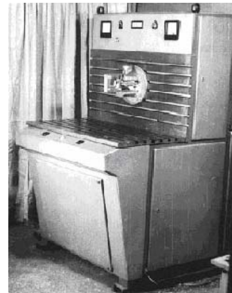
Fig. 1. The technical equipment created in the National Technical University «Kharkiv Polytechnic Institute» (Ukraine) for processing of the tubular work-pieces: a) it is the massive single turn INDUCTOR; b) it is the MAGNETIC PULSED INSTALLATION MIU-24 (the stored energy is ~ 24 kJ)
