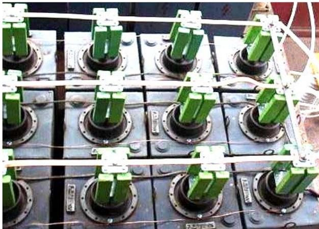
Fig. 25. General view of a fragment of a powerful high-voltage CES single module performance at a rated voltage of  $\pm 50$  kV and rated stores electric energy 420 kJ with its parallel-connected capacitors type ИК-50-3 in the amount of 112 pieces. and rigidly mounted on their findings of high-volume constant high voltage protective graphite-ceramic resistors TBO type-60-24  $\Omega$  [49]
