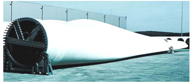
Fig. 8. Enlarged image of a single blade of the length of 40 m of modern horizontal-axis wind turbine, located on the plant site of the finished product [2, 11]
