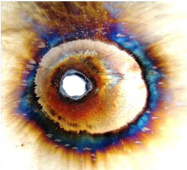
Fig. 12. External view of the area with a diameter of about 12 mm of penetration through the flat wall TS steel roof ( h=1 mm; h_a=14 mm) by a direct action on long-term C- component of the current artificial lightning and rounded zone diameters up to 58 mm in its surface melting from direct action on TS of pulsed A- components of with standardized requirements for [3, 4] ATP
