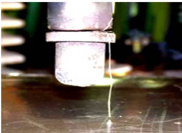
Fig. 4. General view of the TES with copper EEW desktop of generators PCG-A and PSG-C when tested in their discharge circuits TS thin steel roof on electrothermal resistance to direct impact on them of pulse A- and long-term C- artificial lightning current components with a normalized according to [3, 4] ATP ( l_e=37-50 mm) [8]
