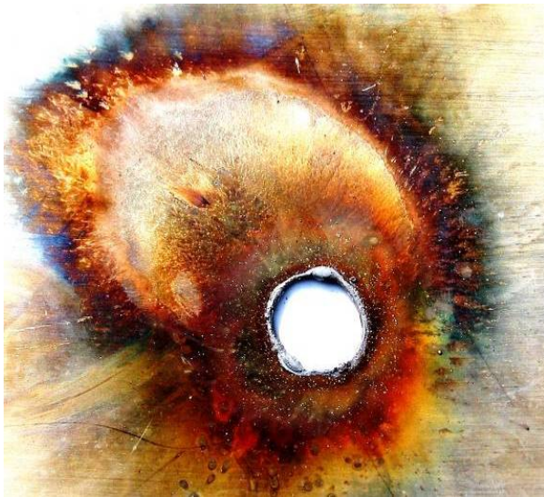
Fig. 15. External view of rounded zones of thermal influence on the flat roof of the TS steel of pulsed A - and long-term C - artificial lightning current components with standardized requirements for [3, 4] ATP accompanied keyhole TS wall ( h=1 mm; h_a=14 mm)
