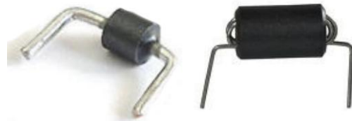
Fig. 2. Miniature Filters Built Based on Ferrite Elements (FE) and Designed for Installation on a Printed Circuit Board
