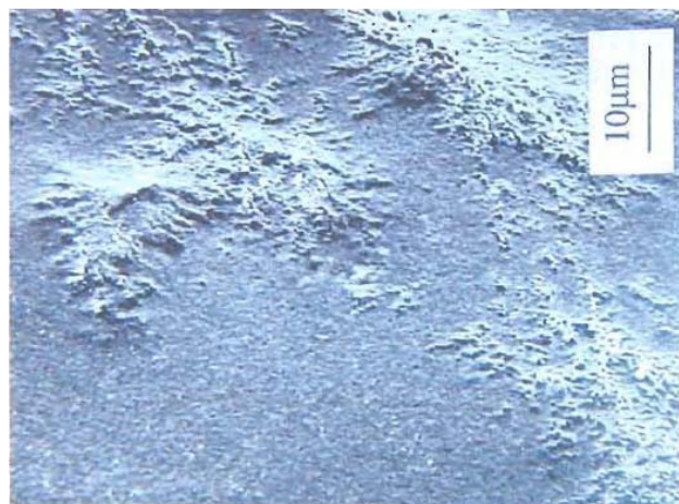
Fig. 1. Photo of emerging water treeing in cross-linked polyethylene insulation of power cable, obtained by power electron microscope [4]
