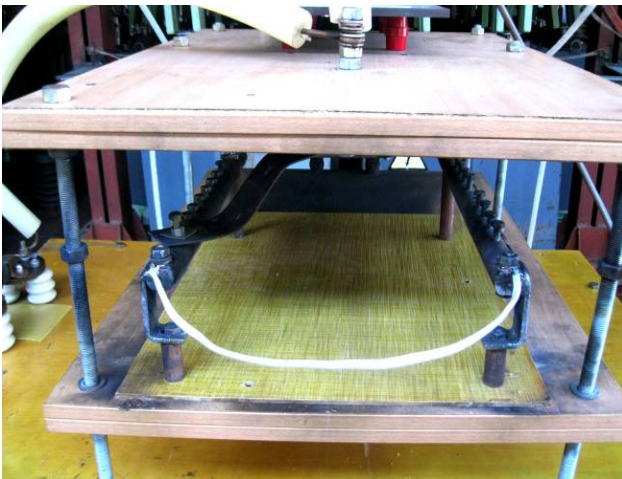
Fig. 8. View of the working table of the generator ГИТМ-10/350 with rigidly fixed on its massive steel electrodes with solid round copper conductors of the total section of S_1 \approx 5 \text{ mm}^2 of the TS of the wire ПНП 2×2,5 with a PVC insulation of the length of 0.5 m to the impact on them aperiodic current pulse 15/335 \mu\text{s} of the artificial lightning of amplitude of about I_{mL} \approx 85.6 \text{ kA} ( U_{31-3} \approx 16.5 \text{ kV} ; U_{34} \approx 4.2 \text{ kV} )
