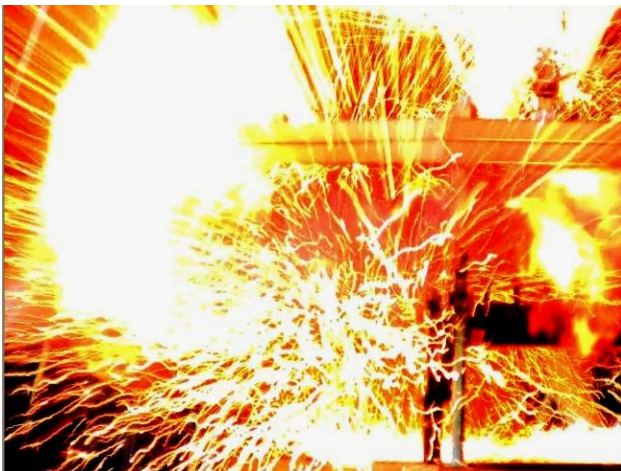
Fig. 5. The initial stage of EE of the copper conductor with cross-section of S_1 \approx 3.2 \text{ mm}^2 of the TS of the RF coaxial cable PK 50-7-11 with a solid PET insulation of the length of 0.5 m in the high-current discharge circuit of the generator ГИТМ-10/350
