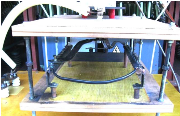
Fig. 10. View of the working table of the generator ГИТМ-10/350 with rigidly fixed to its massive steel electrodes solid circular core section of the TS of the continuous circular aluminum АППВНг2×6 conductor of the cross section S_1 \approx 6 \text{ mm}^2 of the wire with PVC insulation length of 0.5 m before exposure by the aperiodic current pulse 15 / 335 \mu\text{s} of the artificial lightning of amplitude of about I_{mL} \approx 85.6 \text{ кА} ( U_{31.3} \approx 16.5 \text{ кV} ; U_{34} \approx 4.2 \text{ кV} )
