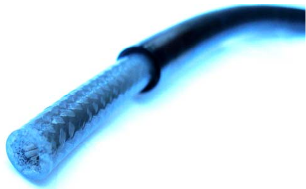
Fig. 6. View of the end cutting of the TS of the RF coaxial cable PK 50-7-11 with a solid PET insulation of the length of 0.5 m after passing on his split round copper conductor of the cross-section of S_1 \approx 3.2 \text{ mm}^2 of the test current impulse 17/310 \mu\text{s} by the artificial lightning from the generator ГИТМ-10/350 and its EE with complete sublimation of copper ( I_{mL} \approx 82.9 \text{ kA} ; \delta_{m1} \approx I_{mL}/S_1 \approx 25.9 \text{ kA/mm}^2 ; \tau_f \approx 17 \mu\text{s} ; t_m \approx 28 \mu\text{s} ; \tau_p \approx 310 \mu\text{s} ; J_L \approx 1.76 \cdot 10^6 \text{ A}^2 \cdot \text{s} ; q_L \approx 37.9 \text{ C} )
