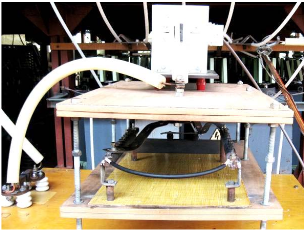
Fig. 4. The view of the working table of the generator ГИТМ-10/350 with rigidly fixed to its massive steel electrodes split round copper conductor with cross-section S_1 \approx 3.2 \text{ mm}^2 of the TS of the RF coaxial cable PK 50-7-11 with a solid PET insulation of the length of 0.5 m and «plugged» with electrothermal tests its braided copper shield-up exposure to the aperiodic current pulse 15/335 \mu\text{s} of the artificial lightning amplitude of about I_{mL} \approx 85.6 \text{ kA} ( U_{31-3} \approx 16.5 \text{ kV} ; U_{34} \approx 4.2 \text{ kV} )
