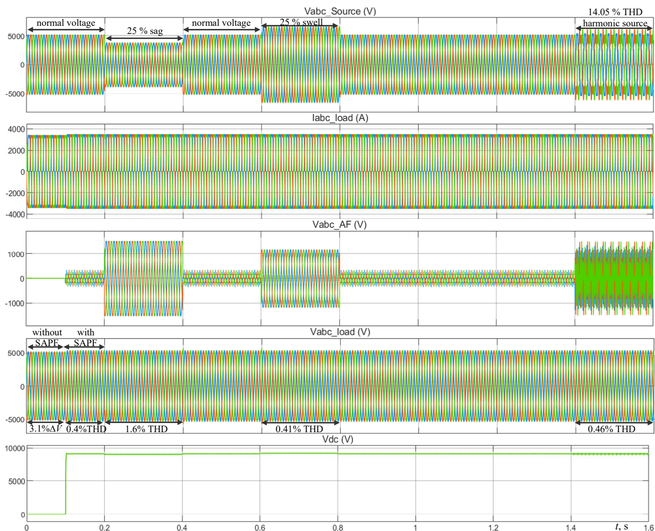
Fig. 13. Voltage waveforms and load current scenario 1
