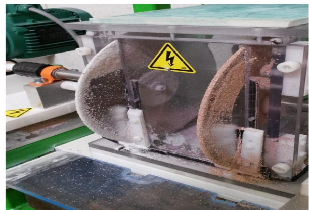
Fig. 2. Collection of insulating particles in the two-rotating-disk tribo-aero-electrostatic separator
