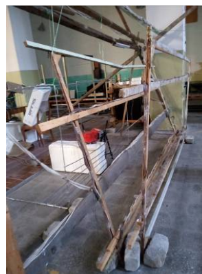
Fig. 12. Two compensating windings of active shielding system
