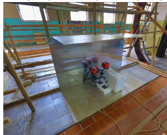
Fig. 6. Passive shield without side plates
