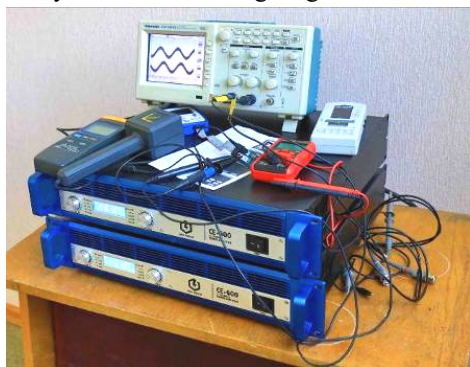
Fig. 7. Power amplifiers for powering compensation windings
