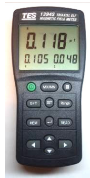
Fig. 9. Three-coordinate magnetometer for measuring resulting magnetic field
