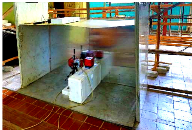
Fig. 11. Experimental installation of passive shield with side plates
