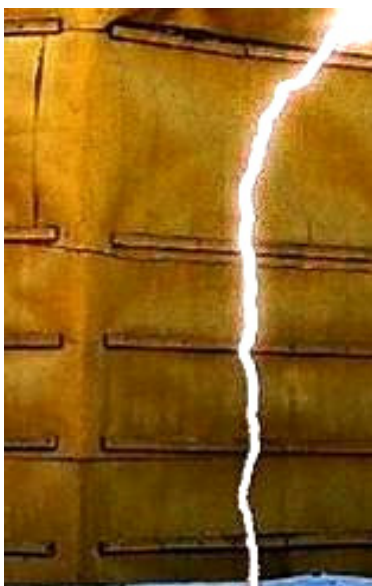
Fig. 7. General view of a zigzag cylindrical plasma channel of a spark discharge with almost spherical zone of radius r \approx x_i of active impact ionization of air, which glows brightly at the top near the potential electrode of the DEDS «tip-plane», during the electrical breakdown of its air gap by a switching aperiodic high-voltage pulse of the time shape T_m/T_p \approx 200 \mu\text{s}/1990 \mu\text{s} of positive polarity ( l_{\min} = 1,5 \text{ m} ; U_e(t) \approx U_d \approx 611,6 \text{ kV} [27])
