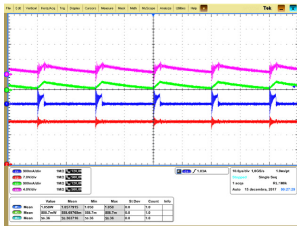
Fig. 8. Measured time waveforms of voltages and currents for the single-phase buck-boost converter in buck mode with 1 W input power
