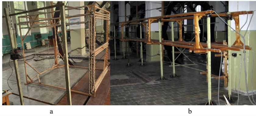
Fig. 4. Laboratory installation for the study of the complex effect of PL+TS, created on the magnetic measuring stand of the IEMS NAS of Ukraine (a – physical model of a low-voltage busbar of the TS, 150 A; b – physical model of the PL 150 A)
