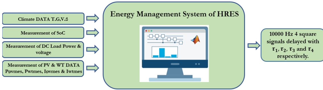
Fig. 2. Block diagram of the energy management system
