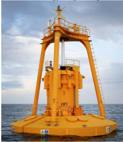
Fig. 3. OPT © power buoy device serves as a typical illustration of a self-reacting point absorber [10]
