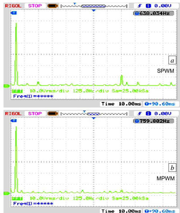
Fig. 12. Measurement of THD using the oscilloscope's FFT tools: a – THD of SPWM; b – THD of MPWM
