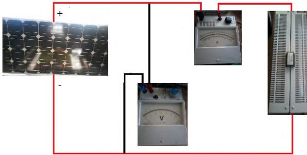
Fig. 13. Circuit measurement of  $I_{pv}(V_{pv})$  and  $P_{pv}(V_{pv})$  of STP080S-12/Bb module
