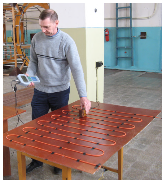
Fig. 10. Study of the distribution of MF flux density of the EHCS laboratory model with a coaxial HC of the «VOLTERM» type on the magnetometer stand of IPMach of the National Academy of Sciences of Ukraine
