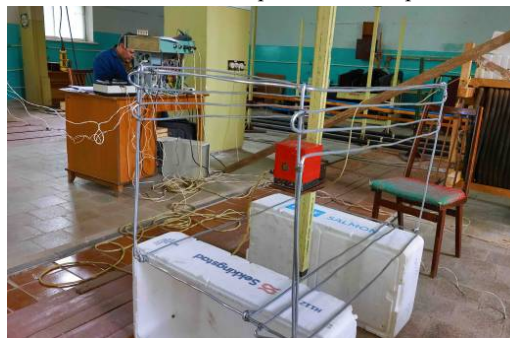
Fig. 7. The multi-circuit passive shield and the control system of the experimental setup of multi-circuit passive and active shielding
