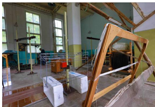
Fig. 6. The compensation winding and multi-circuit passive shield of the experimental setup
