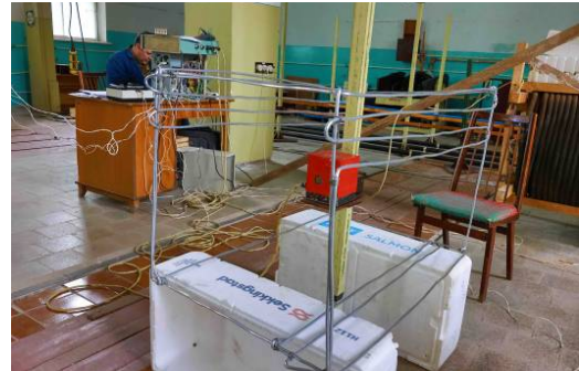
Fig. 7. The multi-circuit passive shield and the control system of the experimental setup of multi-circuit passive and active shielding
