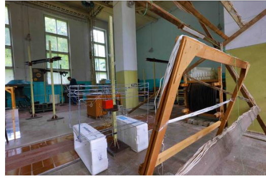
Fig. 6. The compensation winding and multi-circuit passive shield of the experimental setup
