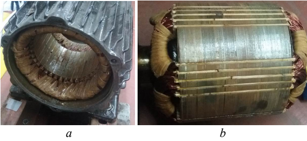
Fig. 11. Active part of the armature (a) and rotor (b) of the ISEM experimental sample
