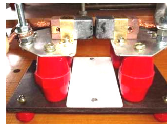
Fig. 3. General view of the high-voltage two-electrode high-current air commutator F_2 with graphite electrodes of a rectangular shape for nominal constant voltage of \pm 5 kV and charge q_L up to \pm 300 C, which is placed in the discharge circuit of a powerful LCG of the UITOM-1 type [16]
