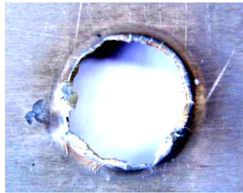
Fig. 16. General view of the inner rounded zone of the through burning of the sheet TS during the lightning resistance test of the AC cladding of the aluminum alloy of the AMr2M brand with thickness of h = 1 mm from the combined action on it in the discharge circuit of a powerful high-voltage PCG of the UITOM-1 type of pulse A - and long-term C - components of the full current of artificial lightning with normalized ATP
