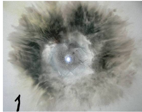
Fig. 17. General view from the side of the anchoring zone of the results of through burning on the outer surface of the TS of the flat duralumin panel with thickness of h=1.2 mm of the fuel tank lining of the domestic aircraft «An» of the plasma channel simulated in the discharge circuit of a powerful high-voltage PCG of the UITOM-1 type of artificial thunderstorm discharge with radius r_e \approx 3.7 mm of its wall from the direct action of normalized A - I_{mA1} \approx 199.5 kA; t_{mA1} \approx 42 \mu s; \tau_{p1A} \approx 500 \mu s; J_{aA} \approx 1,99 \cdot 10^6 J/ \Omega ), B - ( I_{mB} \approx 6.16 kA; I_{cB} \approx 2220 A; q_{LB} \approx 11.1 K; \tau_{p1B} \approx 5 ms) and C^* - ( I_{mC^*} \approx 1112 A; \tau_{p1C^*} \approx 13.6 ms; q_{LC^*} \approx 5.79 K; I_{cC^*} \approx q_{LC^*}/\tau_{p1C^*} \approx 426 A) components of the full pulse current of artificial lightning (damage area 1A ) [17]
