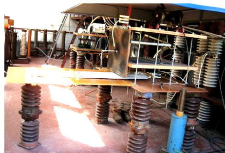
Fig. 5. General view of the improved powerful high-voltage LCB of the UITOM-1 type (in the foreground is a work table with a three-electrode switch F_1 for nominal constant voltage of \pm 50 kV and an air extraction system, and in the background is an individual high-voltage powerful generators GIC-A (GIC-D), GIC-B, GIC-C and GIC-C*)
