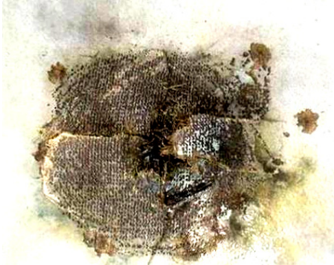
Fig. 18. General view of the damage zone with diameter up to 100 mm with through burning in sheet TS with thickness h=2.9 mm of the experimental composite cladding of the aircraft, tested for lightning resistance in the discharge circuit of a powerful high-voltage PCG of the UITOM-1 type, when it is directly affected by only the pulse A - component of the artificial lightning current with normalized ATP ( I_{mA1} \sim 212 kA; t_{mA1} \sim 32 \mu s; \tau_{p1A} \sim 500 \mu s; J_{aA} \sim 2.11 \cdot 10^6 J/ \Omega ) [16]
