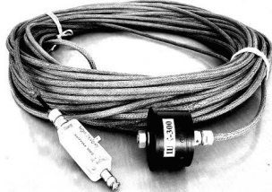
Fig. 11. General view of a high-voltage measuring shunt of the ShK-300M type, connected to the input of an additionally shielded radio-frequency coaxial cable of the RK 75-7-11 brand l_c \approx 70 m long, the output of which is connected to the input of the SPN-300 shielded matching voltage divider with two output coaxial 1:1 and 1:2 connectors for the coordinated connection of the measuring channels of three DSOs to them (for example, Tektronix TDS 1012 series) with simultaneous registration in the discharge circuit of a powerful UITOM-1 type PCG at once of three components of the full pulse current of artificial lightning with different ATPs [16]
