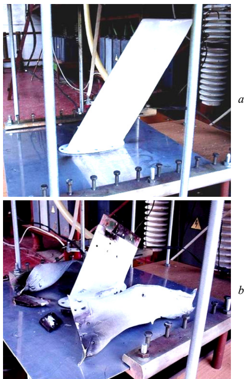
Fig. 19. General view of the experimental model of the aviation receiving-transmitting antenna of the AC before (a) and after (b) direct action on it in the high-current discharge circuit of the modernized powerful PCG of the UITOM-1 type of the pulse A -component of the artificial lightning current with normalized ATP ( I_{mA1} \sim 211.9 kA; t_{mA1} \sim 32 \mu s; \tau_{p1A} \sim 500 \mu s; J_{aA} \sim 2,1 \cdot 10^6 J/ \Omega ) [16]
