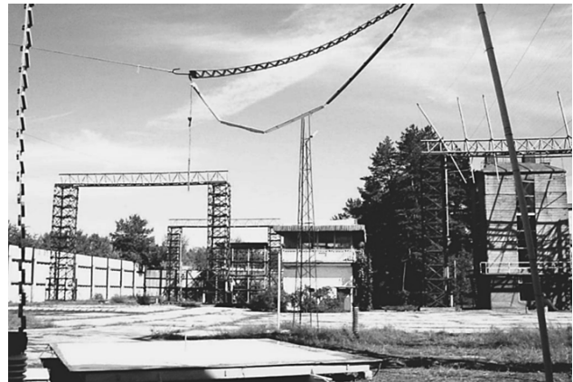
Fig. 2. General view of the ultra-high-voltage air DEES «tip-plane» ( l_{\min} = 3 m), in which to the potential upper steel rod electrode pointed at the lower edge with radius r_0 \approx 15 mm, placed in the center of its grounded lower flat electrode made of galvanized steel with overall dimensions of 5 \times 5 m, OPN-2,5 for nominal electrical pulse voltage of 2.5 MV with the division coefficient K_d \approx 53650 is connected [18]
