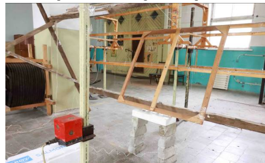
Fig. 6. Compensation winding of the experimental setup
