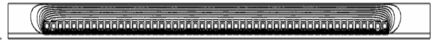
Fig. 10. Distribution of lines of force of the magnetic field in the cross-section of a multi-turn inductor at frequency of 1000 Hz
