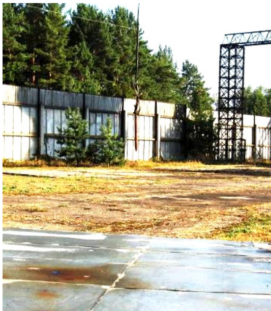
Fig. 2. The general view of the tip-plane air DEES with a discharge gap of length l_{min} = 1.5 m (the tip on a vertically placed steel electrode-rod with a diameter of 30 mm has a radius of rounding of its edge \sim 1 mm; the horizontal plane of the electrode is 5 \text{ m} \times 5 \text{ m} made of thin galvanized steel sheets)
