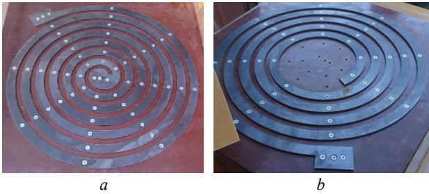
Fig. 5. External view of the PIAPF inductor: the first version (a), the second version (b)
