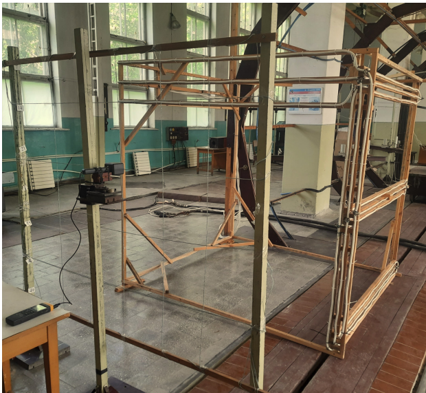
Fig. 9. Full-scale laboratory layout of a low-voltage current conductor of the TS 10/0.4 kV, 100 kVA on the magnetic measuring stand
