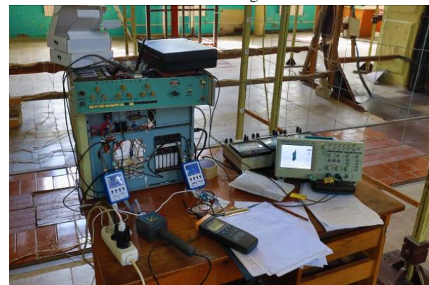
Fig. 6. Double-circuit system of active silencing model
