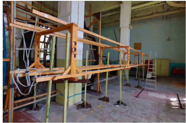
Fig. 4. Power transmission line model with a wire suspension of the «Barrel» type
