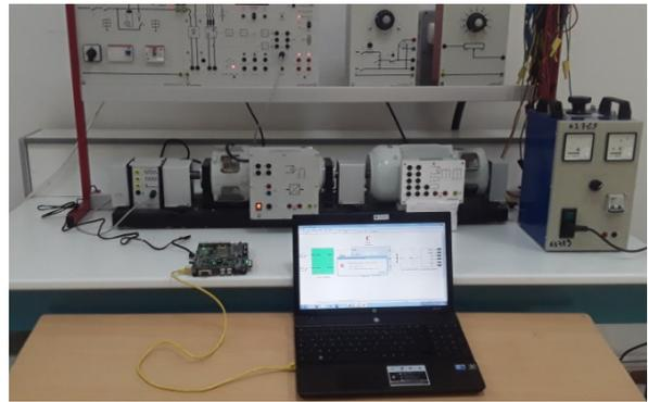
Fig. 22. Fuzzy DTC point to point Ethernet hardware in the loop process
