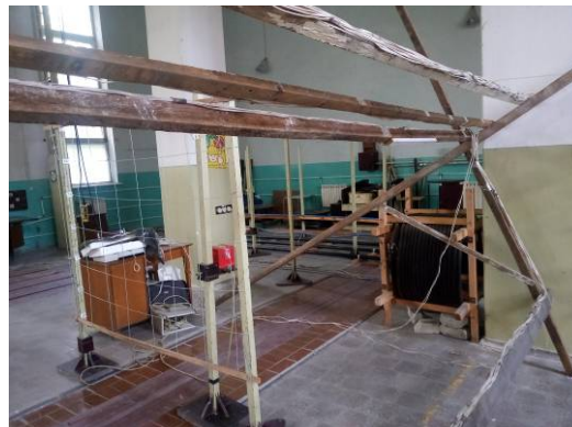
Fig. 5. Model of both canceling windings
