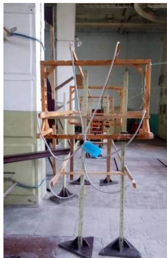
Fig. 4. Model of a two-circuit power transmission line with the arrangement of wires of the «Barrel» type
