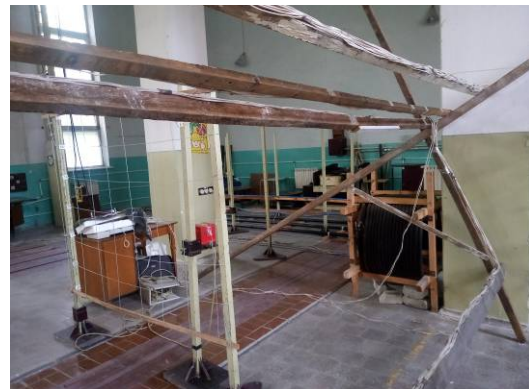
Fig. 5. Model of both canceling windings
