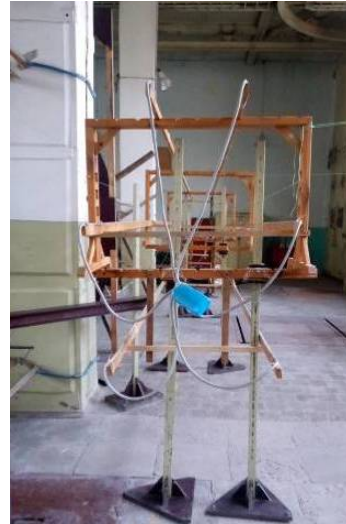
Fig. 4. Model of a two-circuit power transmission line with the arrangement of wires of the «Barrel» type
