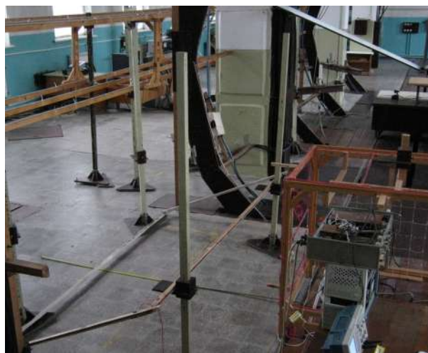
Fig. 13. The layout of the models of power transmission lines, compensating winding and protected area
