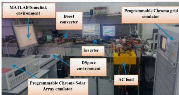
Fig. 1. Depict implemented grid-connected PV system [14]
