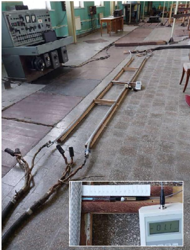
Fig. 8. Experimental installation with a laboratory model of a 330 kV PL's phase and a magnetometer sensor positioning device
